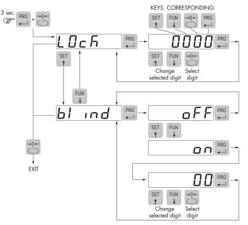
You can select ON / OFF of the parameter BLIND and the setting of a time; the time count starts from the moment when, after exiting the setup menu, the display shows the weight value. After the set time, the display turns off and only a dash appears. This dash cycles through the perimeter of the display counterclockwise. When the display is off, also the 4 keys are disabled, regardless of how you set the keypad lock (LOCK). The only way to access the settings will be PRG + 0.
