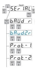
**Modbus:** MODBUS RTU (slave) protocol. used only if PROT-2 is configured equal NONE. See details in the relevant paragraph. Selectable communication patrameters:
