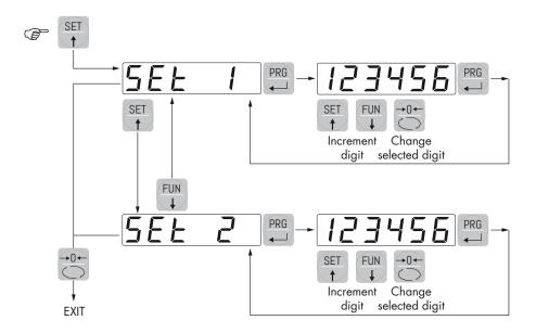
During the step of setting the setpoints, both outputs are disabled. If the setpoint value in memory is 0, the corresponding output is never enabled, regardless of the set-up of the selected setpoints. When the weight is not detectable or out of range, all outputs are disabled (contact open or closed depending on the MODE; see the relevant chapter).
